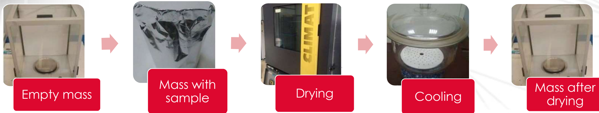
Calcium oxalate monohydrate analysis with moisture balance
