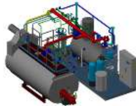
Complete Feed Water Treatment Modules to Boiler connection
