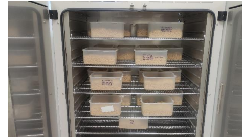
Drying spiked pellets at 35 °C in hepa filtered air flow oven for a week
