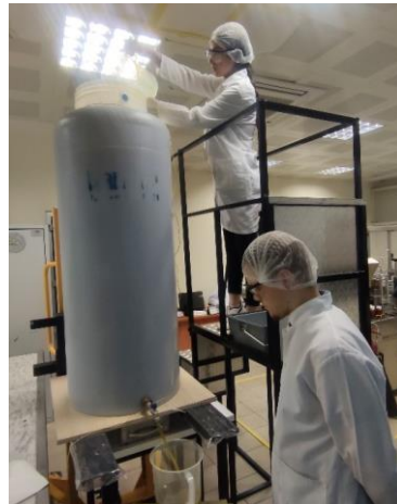
Filling the 320 L container and circulating the content for homogenization
