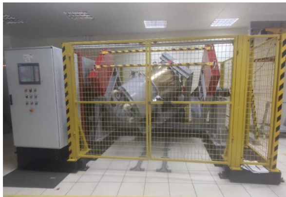
3D homogenization of wood powder (75 kg, 16 hrs)
