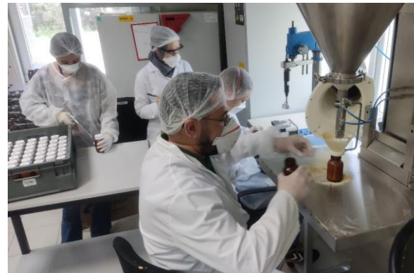
Semiautomatic filling and capping
