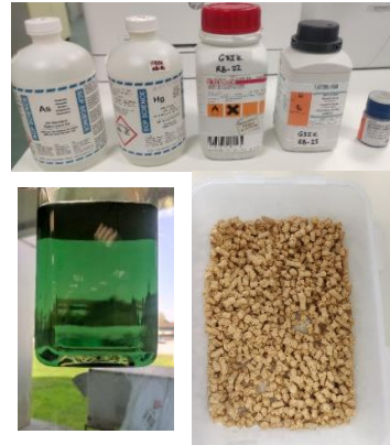
Spiking of elements to pellet (As, Cr, Hg, Pb, Ni)
