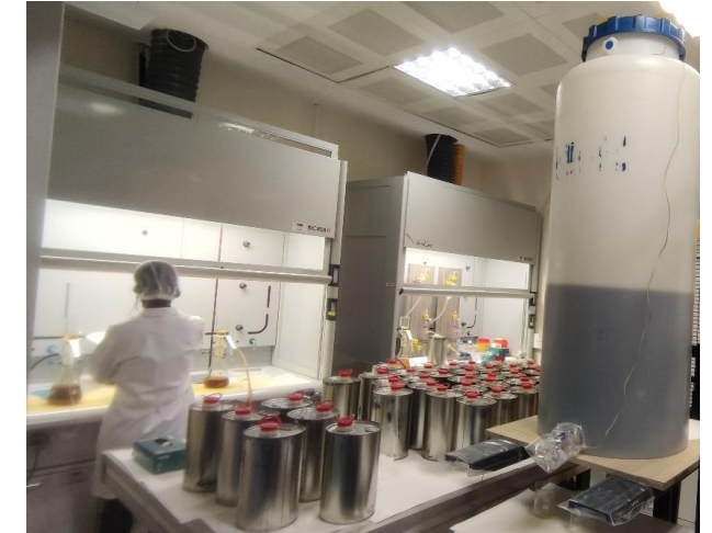
Combining filtered biodiesel in 320 L HDPE container
