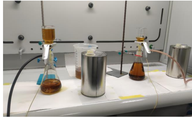
0.7 µm glass fiber vacuum filtering
