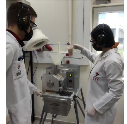
Milling of spiked & unspiked pellets to < 0.5 mm by cutting mill (2 weeks)
