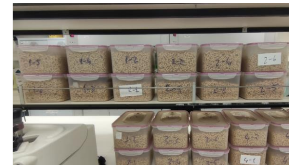
Splitting homogenized material into vacuum containers
