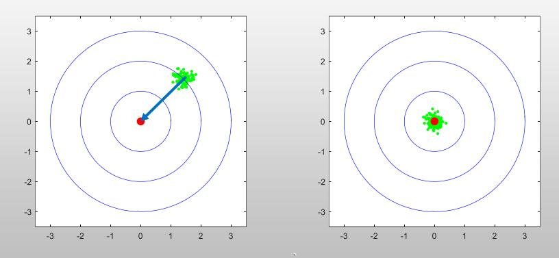
Determine systematic errors by calibration and correct the result
