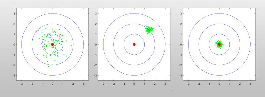
Good accuracy Poor precision Poor accuracy Good precision Good accuracy Good precision
