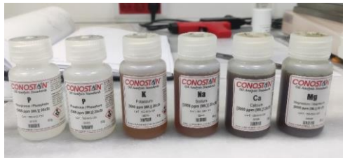
Spiking P, K, Na, Ca, Mg elements in mineral oil
