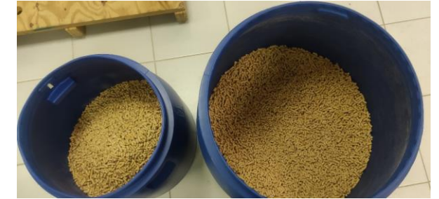
Gentle homogenization by transferring content between 120 L and 60 L HDPE containers
